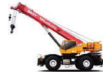
Rough Terrain Crane (25 - 80 ton)
