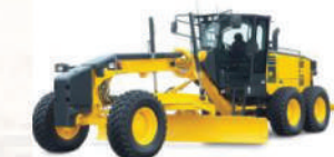
Motor Grader (11.5 - 22 ton)
