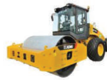
Single Drum Roller (2.5 - 14.5 ton)
